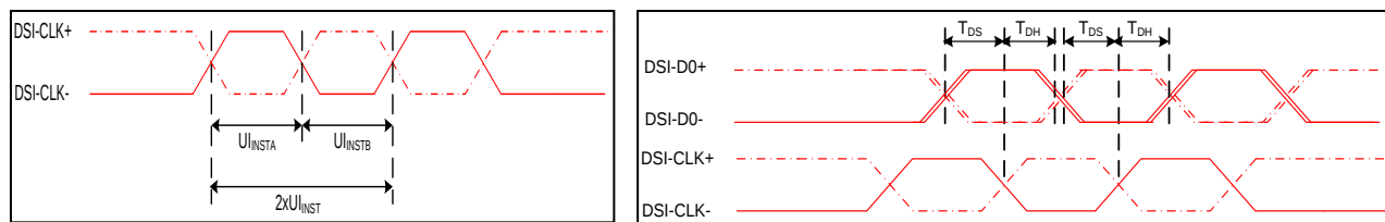
Figure 4 DSI clock channel timing
